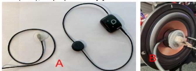
Figure 1 (A): An accelerometer packed in a light-weight silicone (left side) and an AVM prototype (right side). Both sensors have the same accelerometer brand and model. The AVM includes a portable audio digital interface. (B): Setup of both accelerometers attached to the speaker with a double-sided 3M tape.
